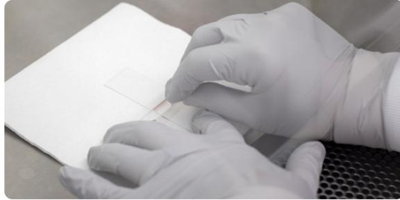
4. Push the top slide forward in a quick, fluid movement, pushing past the end of the slide, making a thin, curved, feathered edge.
